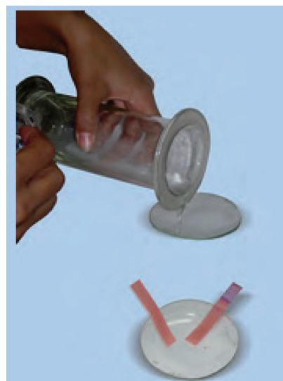
Fig. 24 (b): Testing of solution with litmus papers
